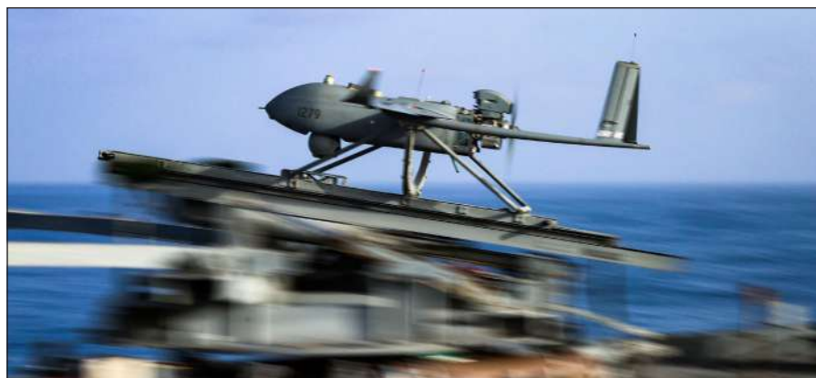
A Textron MQ-19 Aerosonde Unmanned Aircraft system is launched from the expeditionary sea base USS Hershel "Woody" Williams. (U.S. Navy photo)
