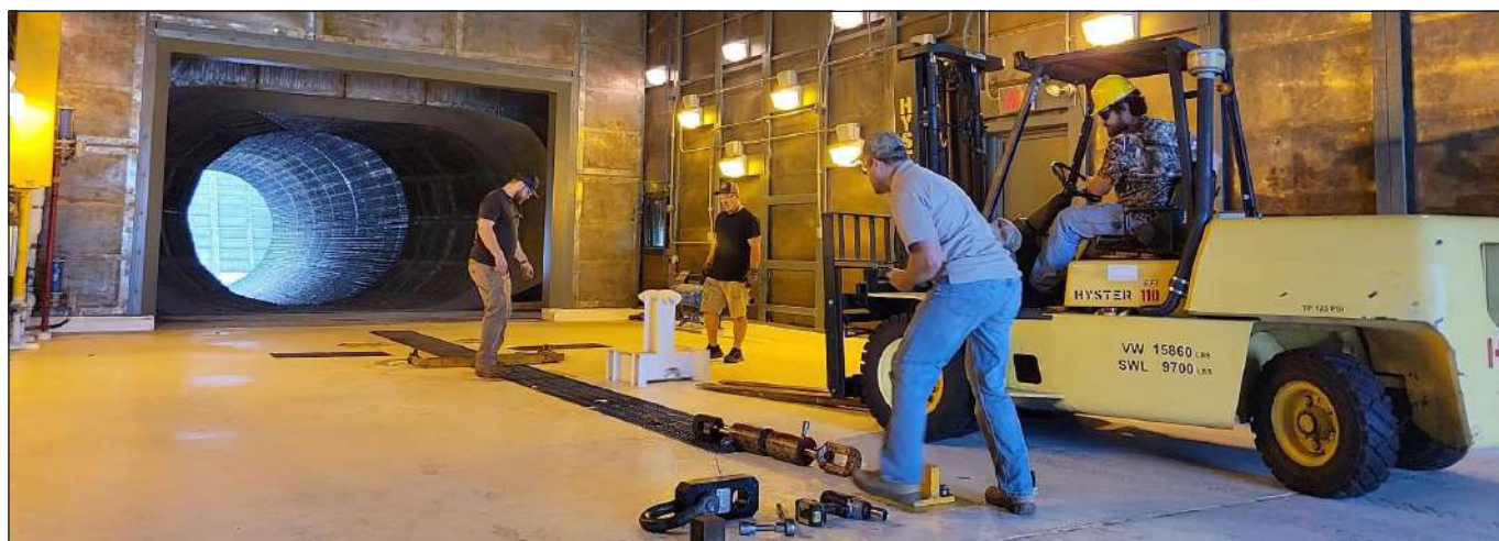
Navy team members facilitate instrumentation setup during a recent load test as part of the collaborative effort between the Common Aviation Support Equipment program office (PMA-260) and Naval Facilities Engineering Systems Command (NAVFAC) to revitalize the T-10 Test Cell Facility that will enable engine testing in a noise-suppressed environment at Naval Air Station Patuxent River, Md. (U.S. Navy photo)
