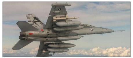
The Next Generation Jammer Mid-Band (NGJ-MB) team recently won the Naval Air Systems Command (NAVAIR) Edward H. Heinemann Award for implementing a critical design change to the NGJ-MB pod by removing the Aft Pivot Assembly (APA) from the pod design, saving millions of dollars and hundreds of hours in testing, and fielding the capability.
